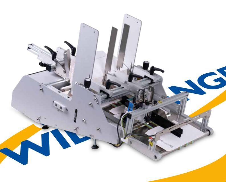
WR FEEDER is a friction feeder for sheets, cards, cases, and coupons up to a maximum size of 250x300 mm. in the 250 version or 400x300 mm. in the 400 version or 500x300 mm. in the 500 version. Thanks to its powerful stepper motor, it can reach a feed speed up to 70 meters/minute.
