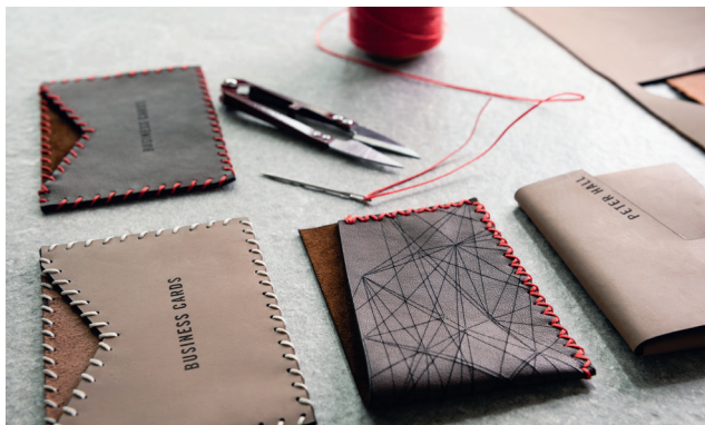
Clean and perfectly sealed laser cut edges of leather incl. engraved details
