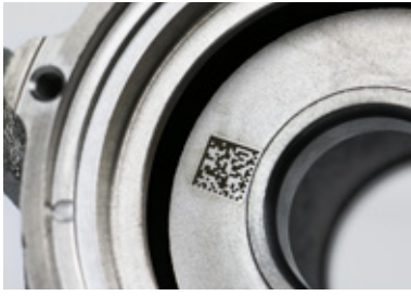
Perfectly readable codes on automotive parts
