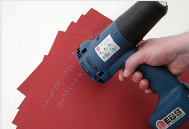
→ Leather (imitation) printed with blue pigmented ink (MEK).
