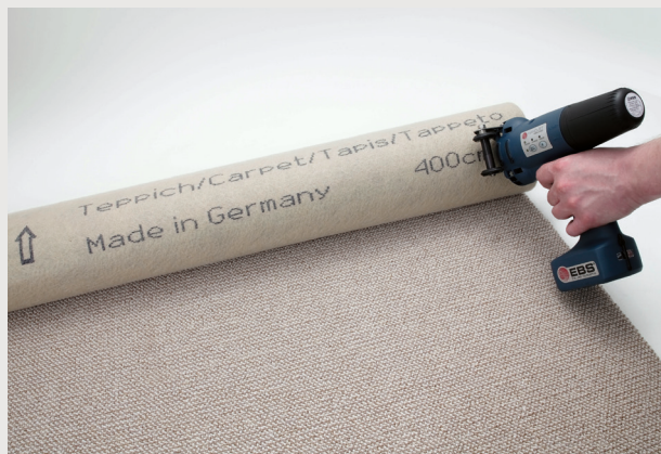
→ Carpeting printed with black universal ink (ethanol); 4-wheel stabilizer.
